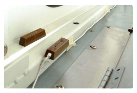
Figure 6. The magnetic sensors are mounted to the test system door.
