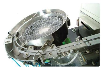
Figure 7. The bowl feeder with the fiber sensors on the test system machine
