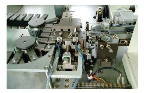
Figure 8. The test system with the fiber sensor, test probes, and slot sensors.
